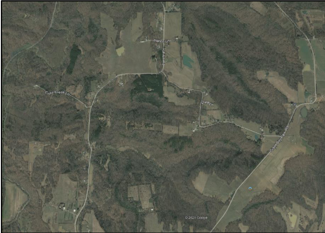
Figure D.27. Mixture of forest and residential structures. Low density WUI intermix. Homes adjacent to forested lands with limited defensible space. Some dead-end spur roads.
