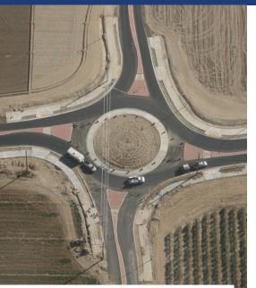
Figure 7. Single lane roundabout in a rural area. Source: Caltrans
