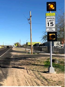
Figure 11. Flashing beacons alerting drivers to decrease speeds in a school zone. Source: FHWA
