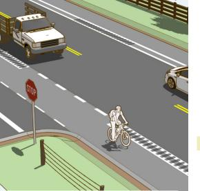
Figure 9. Example of a roadway reconfiguration using available roadway width to include bicycle lanes. Source: Rural Design Guide
